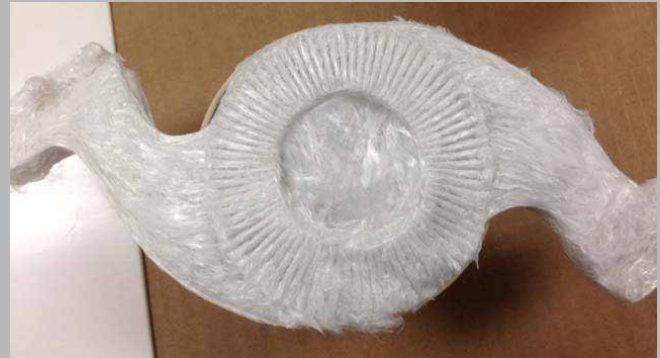
Icon sample after burn out test. (shows glass fiber distribution)
