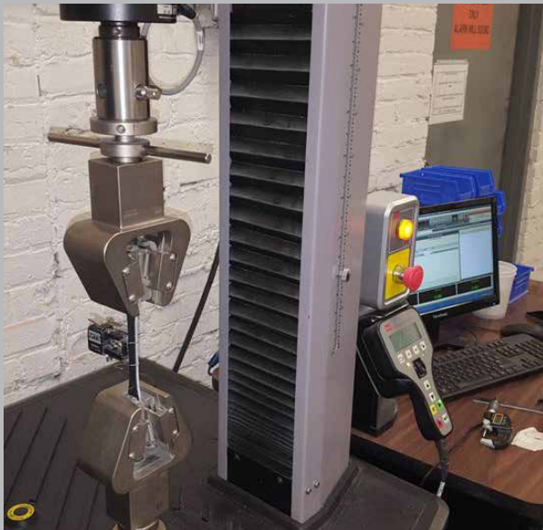
Icon molding material in tensile testing machine
