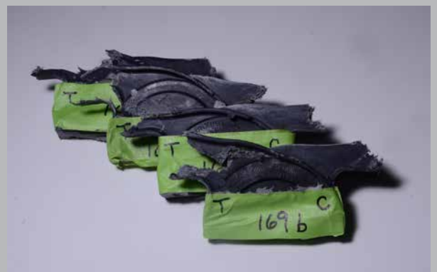
Icon shear test samples showing the predictable mode of failure.
