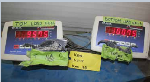
Shear Tested Icons removed from concrete after samples were subjected to ultimate loading criteria.
